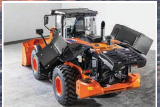
Easy access for maintenance from ground level.
