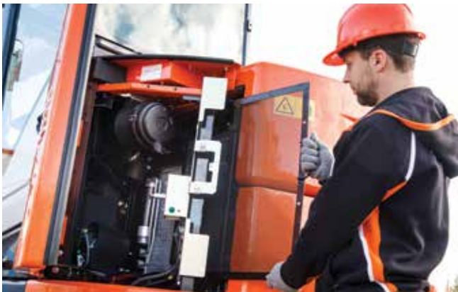
The radiator has a dust-proof net that is easy to clean.
