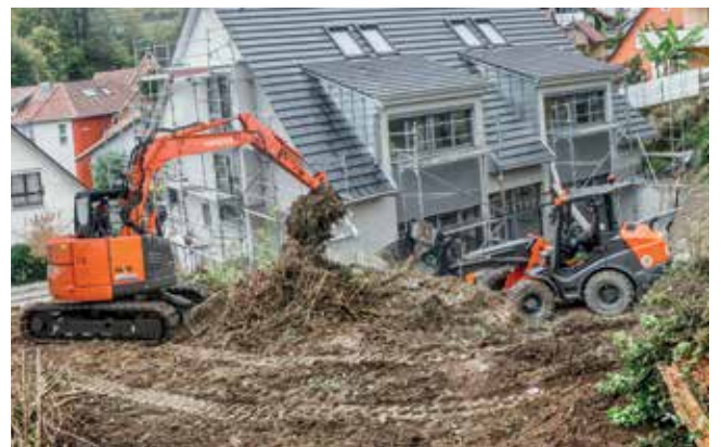
The short-tail swing radius makes the ZX85US-6 ideal for working in tight spaces.
